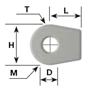
$D = \emptyset 8,1$  H = 22 L = 17 M = Metal T (Thickness) = 10
